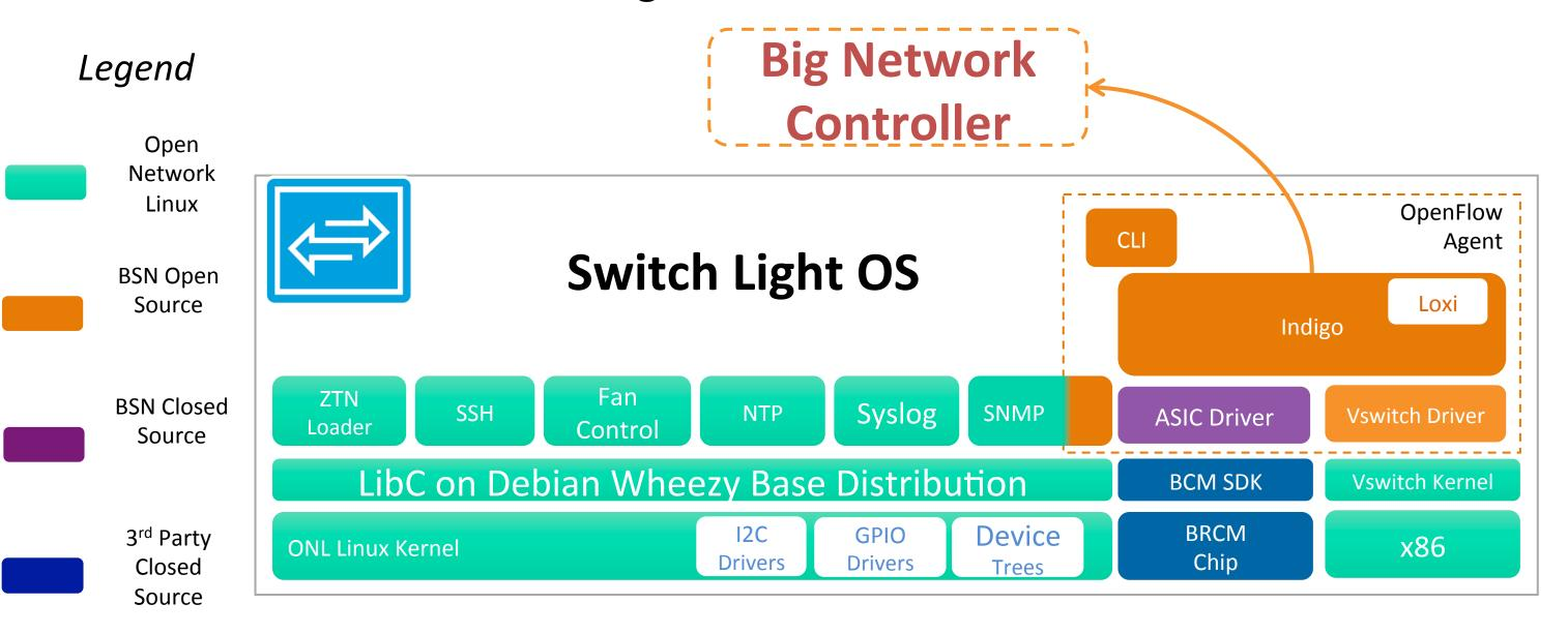
**Switch Light** is our Indigo OpenFlow Agent running on Open Network Linux on x86 or Broadcom hardware.
